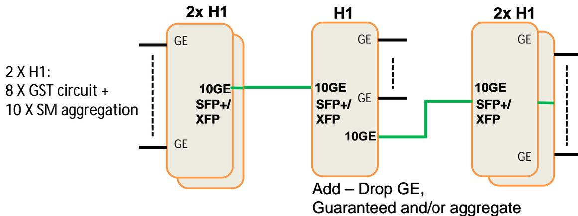
Figure 5, Combining bandwidth-efficient aggregation (SM) and transparent Ethernet line transport (GST) in a transparent Ethernet network. The transparent Ethernet lines can e.g. enable virtual wavelengths, replacing GE transport over wavelengths in an existing WDM network.
