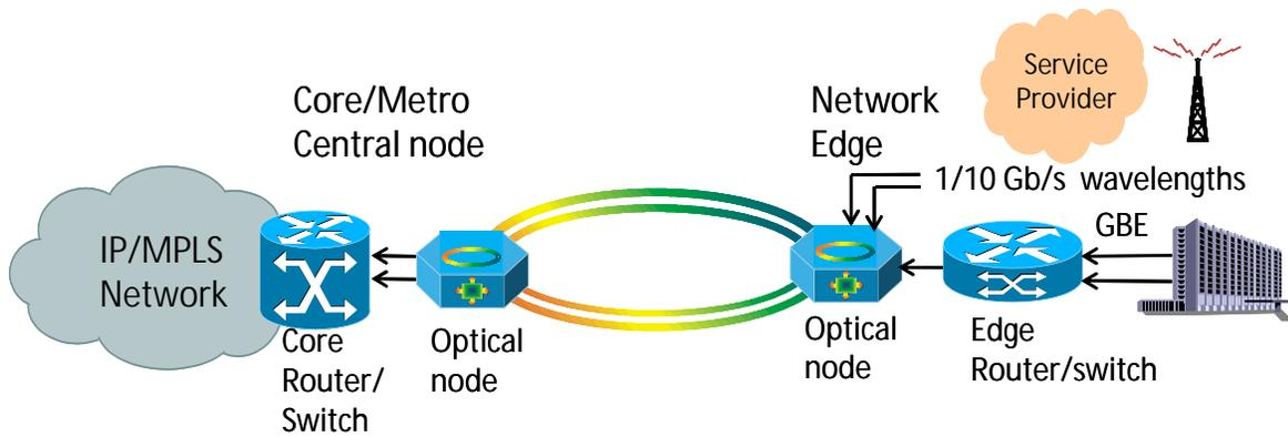
Figure 3, Network with access edge routers or switches and optical nodes for wavelength transport of critical services.
