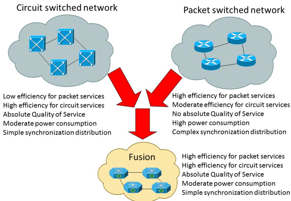
Figure 1, Combining the best properties of circuit and packet switching in the Fusion network.
