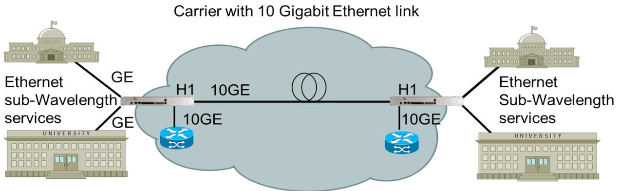
Figure 4, Using TransPacket H1, a 10 Gigabit Ethernet (10GE) wavelength is split into single Gigabit Ethernet sub-wavelengths and offered to customers as Gigabit Ethernet wavelengths with wavelength QoS guarantees. Any leftover capacity on the 10 GE is available for the carriers own transport needs.
