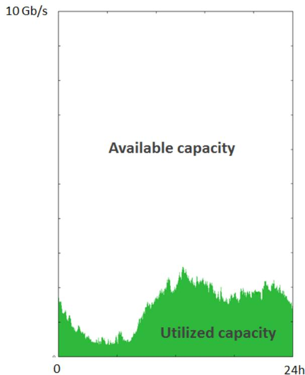
Figure 1: Capacity utilization of a 10GE wavelength during 24 hours on the Trondheim-Oslo link in the network of UNINETT in Norway.
