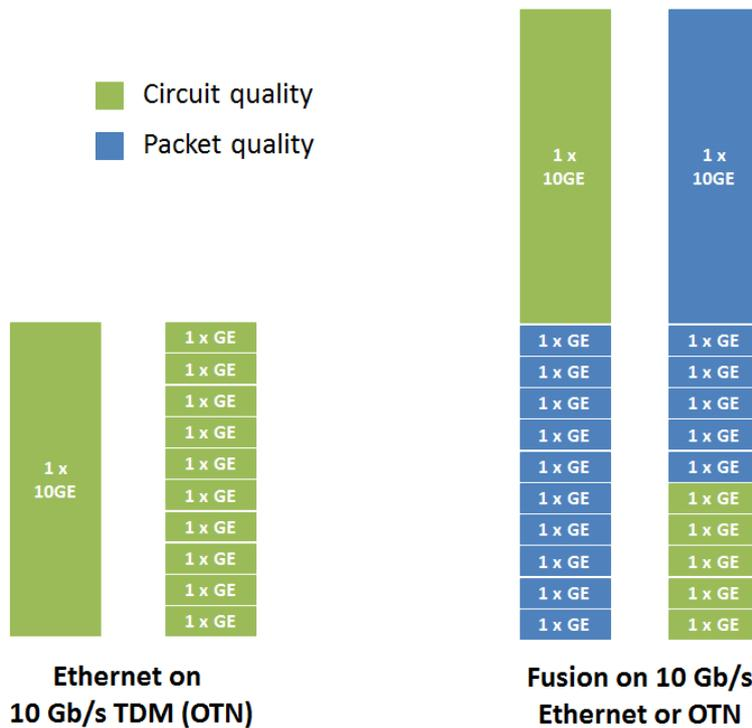
Figure 6, Fusion networking offers the same quality as for circuit switched TDM, but with the added value of offering more interfaces, enabling the same capacity utilization as for packet switched networks.
