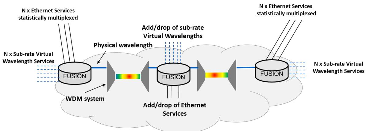
Figure 6, Wavelength service based on offering multiple Ethernet virtual wavelengths of lower rate than the physical wavelength. Additional traffic may be statistically multiplexed into the wavelength through additional Ethernet interfaces of any rate similar or lower than the rate of the physical wavelength. The virtual wavelength approach offers strong OAM capabilities.
