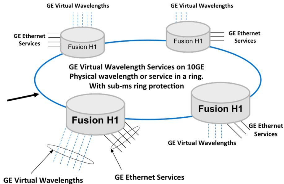
Figure 7, Virtual wavelength services enabled by network applying TransPackets FUSION H1 product.
