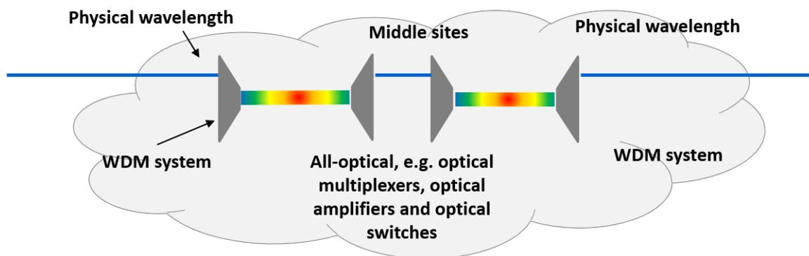
Figure 1: Feeding an alien-wavelength all-optically into a WDM system.
