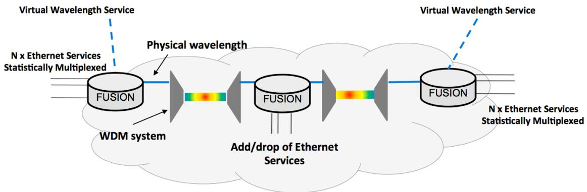
Figure 5, Wavelength service based on a virtual wavelength interface with the same bitrate as the physical interface. Additional traffic may be statistically multiplexed into the wavelength through additional Ethernet interfaces. The virtual wavelength approach also offers OAM capabilities.
