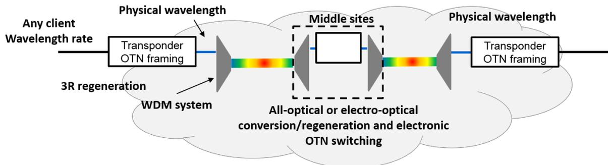
Figure 3, Wavelength service fed through a transponder performing OTN framing, enabling OAM capability. The OTN wavelength may be switched within the network using all-optical switching or using an electronic OTN cross-connect.
