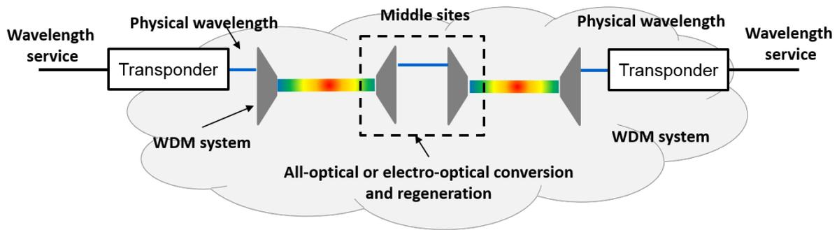
Figure 2, Wavelength service fed through a regenerative transponder into a WDM system.
