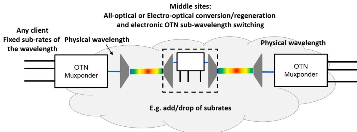
Figure 4, Wavelength service based on “sub-wavelengths” fed through a muxponder performing OTN framing, multiplexing of channels with 1 Gb/s granularity, and OAM. At intermediate nodes in the network, wavelengths and sub-wavelengths may be switched electronically in OTN cross-connects.
